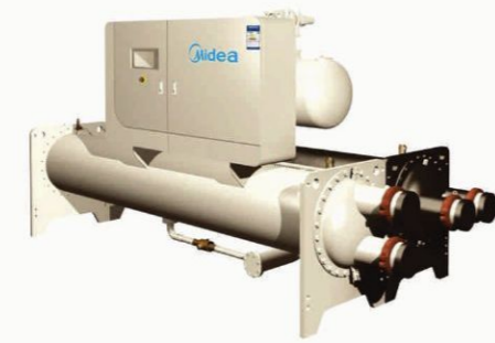
LS B LG XXX - M C F : Screw Chiller R134a, 97~506 RT, COP:5.6~5.9, Flooded R22, 163~560 RT, COP:5.6~5.8, Flooded
